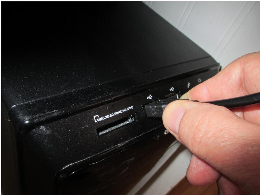
If this is the first time you've attached this device to your computer you will get a message from the operating system notifying you that the device driver is being installed and subsequently that your device is ready for use. You may also be prompted by an AutoPlay dialog box for what application to use with this device (e.g., explore files with Windows Explorer). In this dialog box you will see the volume 'MKIED8B3' naming the HDD you just mounted to your cloning host computer.
