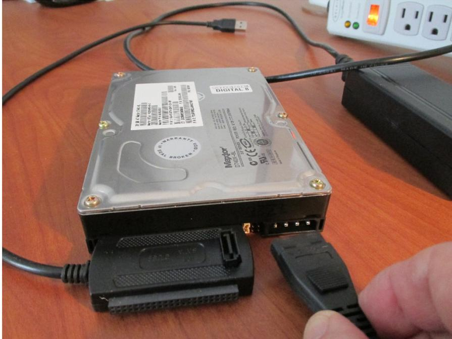
You will hear the drive spin up to speed. Once the drive speed appears to be stable, insert the USB2-IDE cable USB connector in your cloning host computer's USB 2.0 port.
