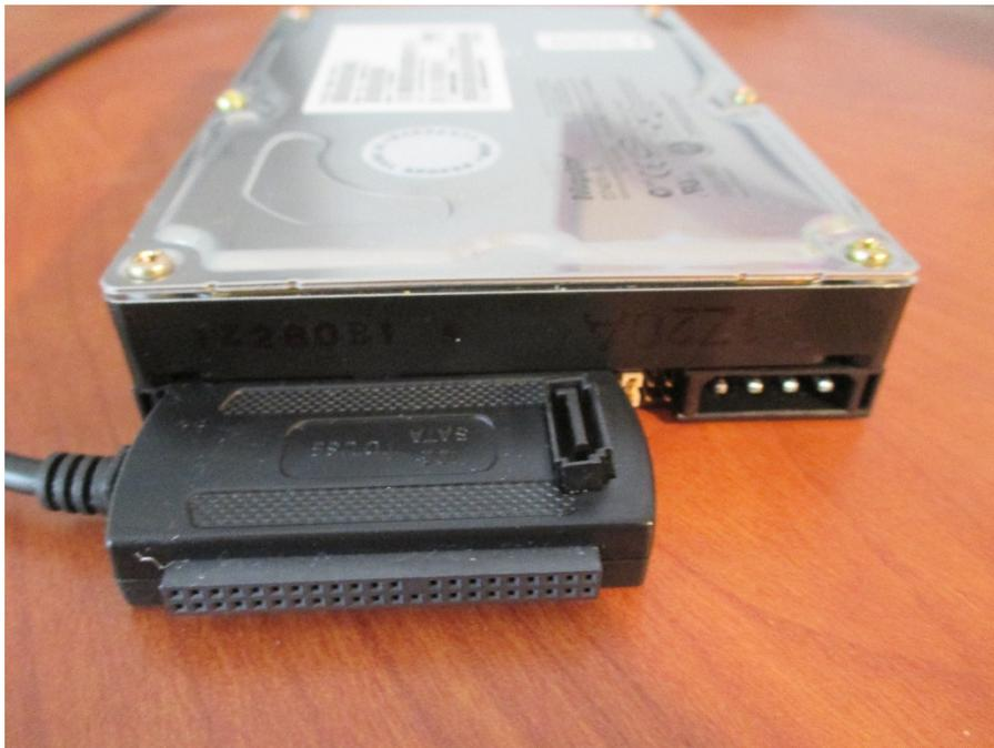
Place the HDD on a flat, sturdy surface where it is secure. Insert the Molex DC power connector from the USB2-IDE adapter into the power connector on the HDD. The Molex 4-pin DC power connector is designed to insert only one way.
