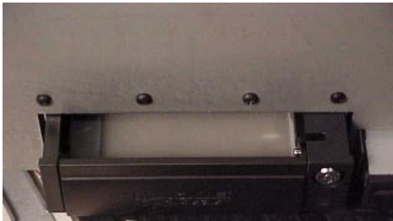
Screws EMI gasket Front view of external hard drive and floppy drive
