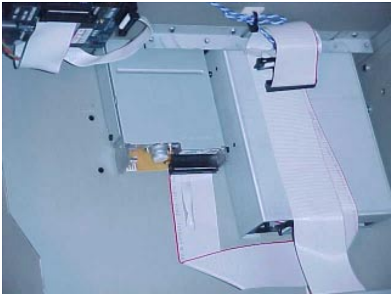
Plate removed, showing the external hard drive and the floppy drive
