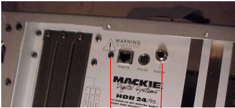
Remove screw and nut to remove the remote board
