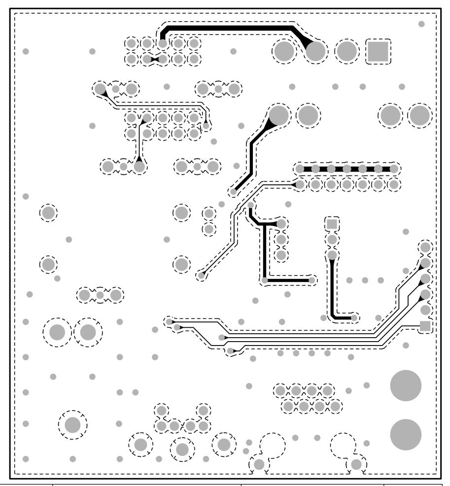
Bottom Surface (Dotted lines are the copper fill)
